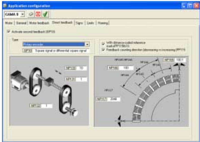
fig. 27 Configuring the application from the WinDDSSetup with the <Direct feedback> label active: Rotary direct feedback with distance-coded I0's.
